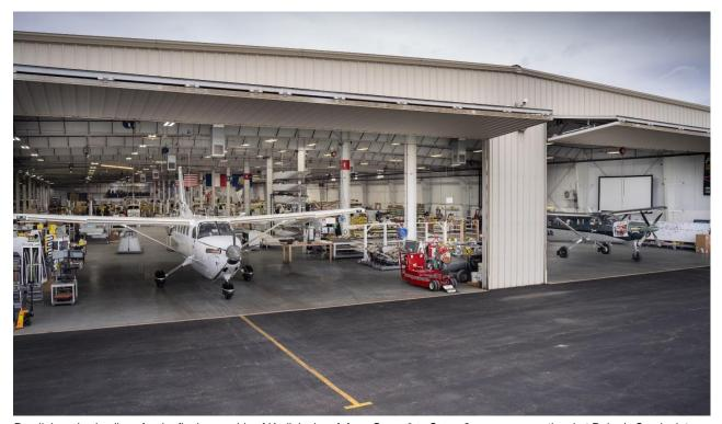
Parallel production lines for the final assembly of Kodiak aircraft from Stage 3 to Stage 6 are now operational at Daher's Sandpoint, Idaho production facility. On the left is the Kodiak 900's final assembly line, while the build-up of Kodiak 100s are completed in a "mirrored" process on the building's opposite side.
