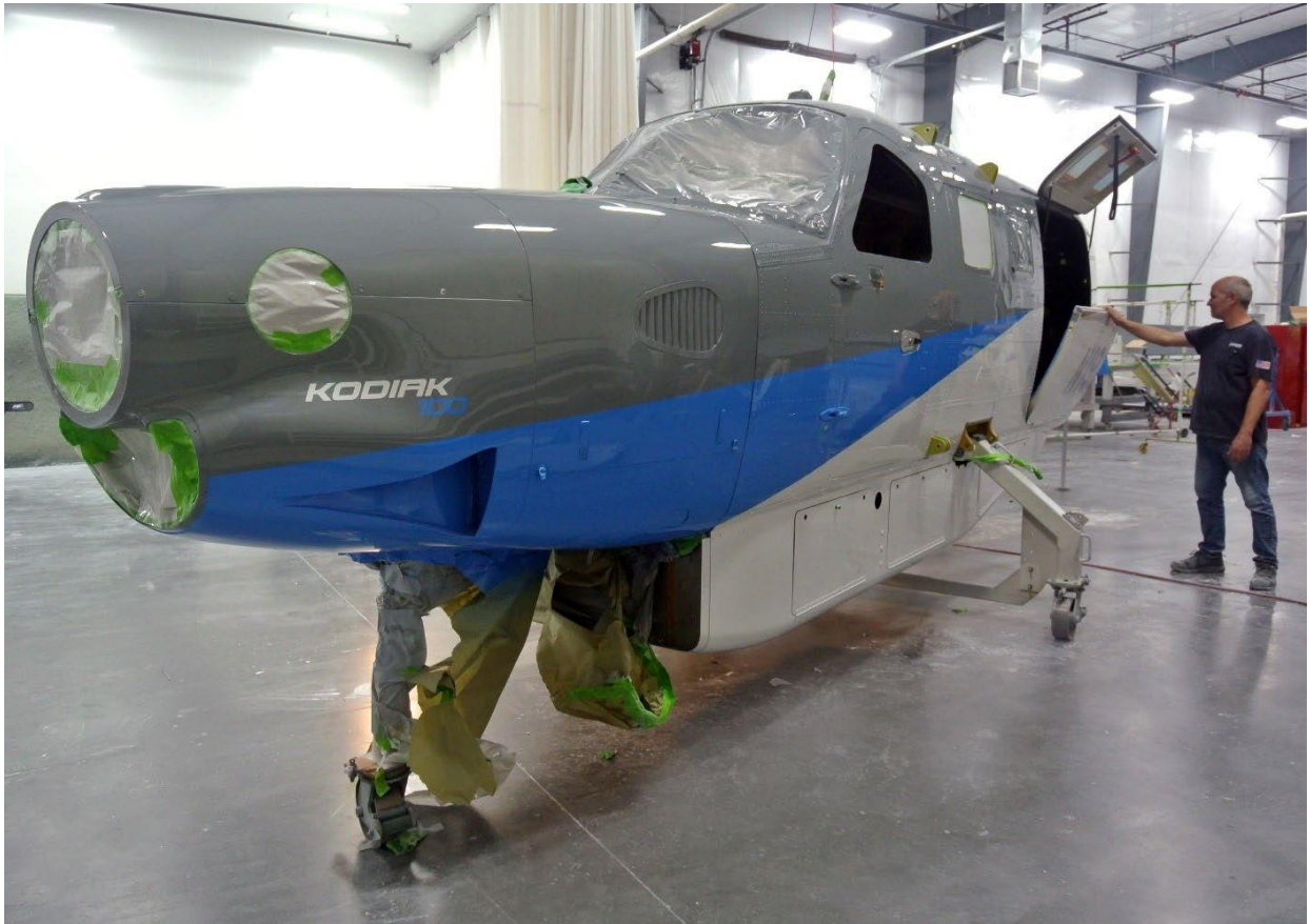
A Kodiak 100 fuselage is inspected after being painted in the new paint facility at Daher's facility in Sandpoint, Idaho.
