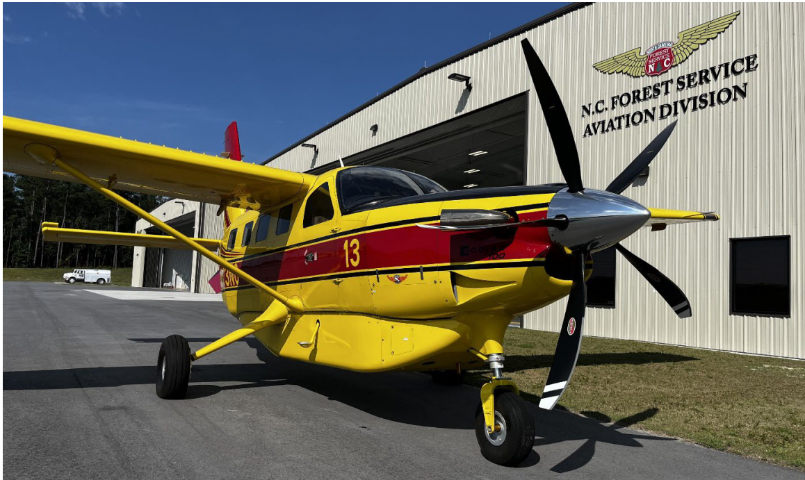
Daher's first Kodiak 100 delivered with a five-blade composite propeller is shown at the North Carolina Forest Service's Aviation Division at Duplin County Airport, Kenansville.
